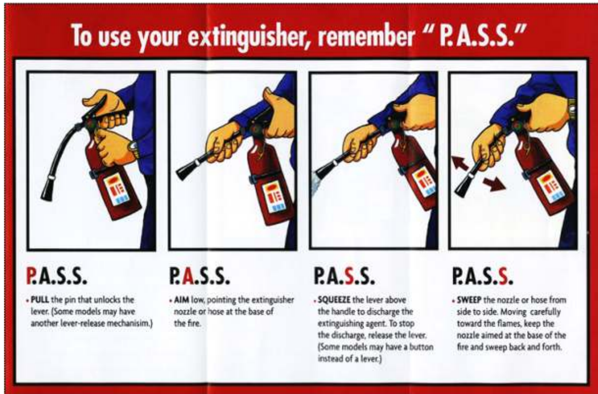
Fig 4.4.2.1 Steps to use the fire extinguisher – use the right extinguisher for the fire
