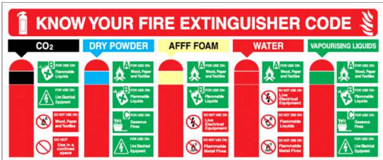
Fig 4.4.1.2 Know your fire extinguisher code
